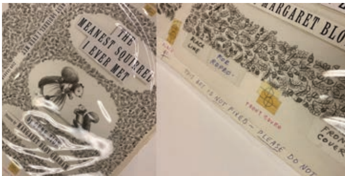
(Left) The plastic overlay on artwork from The Meanest Squirrel I Ever Met is cockled from degradation. (Right) The plastic has shrunk so much that the registration marks no longer align.
