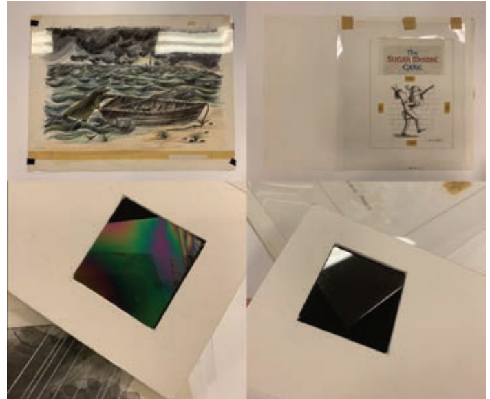
(Top left) Artwork with a transparent plastic overlay from The Storm Book . (Top right) Artwork with a transparent plastic overlay from The Sugar Mouse Cake . (Lower left) Interference colours indicate the plastic is polyester. (Lower right) Absence of interference colours indicate that the plastic is not polyester.
